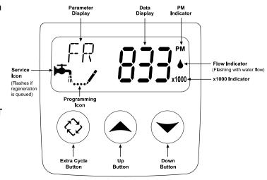
4. Press the Extra Cycle button. Use this display to adjust the Feed Water Hardness. This option setting is identified by "FH" in the upper left hand corner of the screen.
