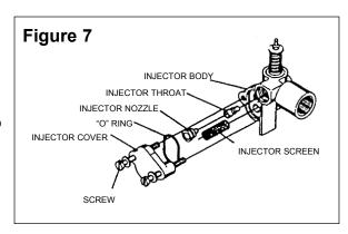
Reassemble using the reverse procedure.
