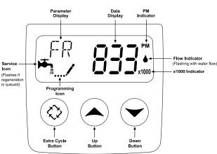
5. Press the Extra Cycle button. Use this display to adjust the Fixed Reserve Capacity. This option setting is identified by "RC" in the upper left-hand corner of the screen.
